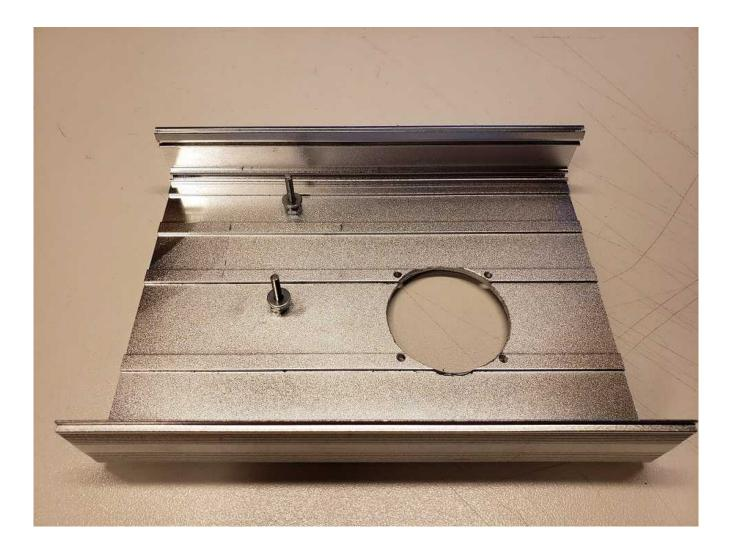
Once holes are located in heat sink mount on case and slide PCB into case to locate Q5 and Q6 mount holes. Mark heat sink centered through holes in PCB. Trill and tap for 4-40 screws. It would be best of you can locate all holes between heat sink fins.
