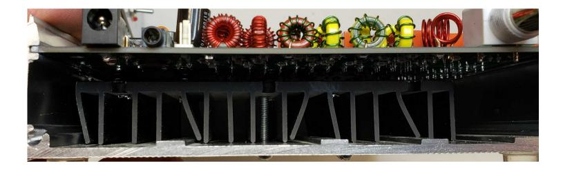
I didn't do this but you could drill some holes under heat sink for natural convection. This an old Pentium Processor heat sink. I wish I could fine a source because it is a perfect fit.
